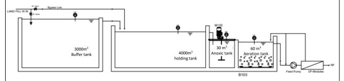
With consideration towards the hydraulic loading, the LTP was designed for 72m³/day (Assume the plant operates at 24hrs), while the effluent quality standards are expected to be compliant with the Kurdish Region of Iraq (KRI) permissible standards for irrigation.
